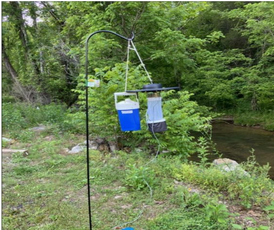
Figure 3.5. CO 2 baited CDC light trap designed to collect questing (host-seeking) female mosquitos.
